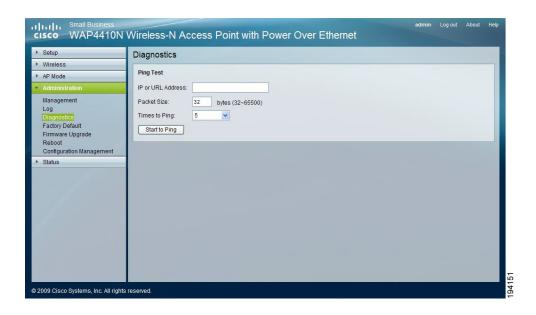
To perform a ping test to help diagnose problems with the access point, follow these steps:
